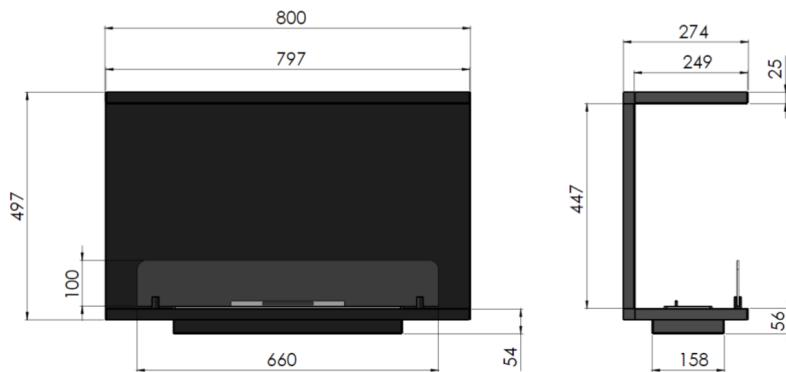
Type/Typ - mounted in the cavity/ do zabudowy we wnęce 800mm x551mm x275mm
